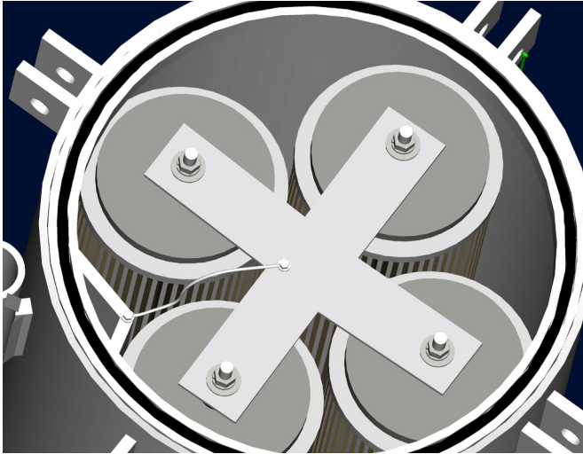
Figure 3. Spider on pre-filter bonded to baffle with braided stainless steel wire.
